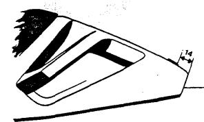
Install decal in the middle of the rear seat tail section, at the correct location.
